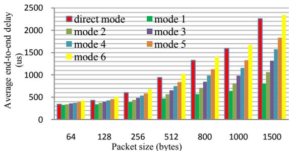
Fig. 3: The average end-to-end delay vs. packet size
