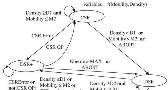
Fig. 2. Principle of mode adaptation in DSR/CSR.
