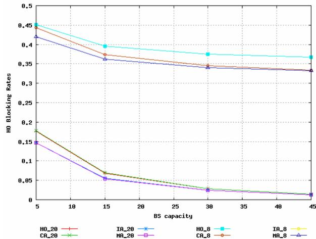
Figure 9: HO Blocking Rates as a function of the BS Capacity
