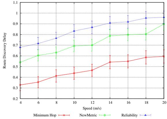
Fig. 5. Route Discovery delay vs Nodes Speed
