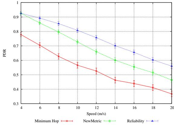
Fig. 4. Packet Delivery Ratio vs Nodes Speed
