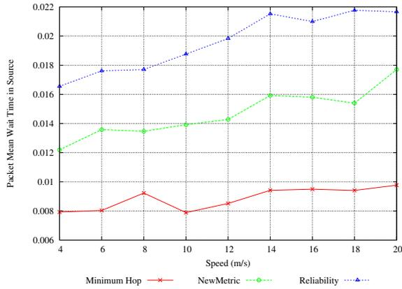
Fig. 6. Mean wait time of packets vs Nodes Speed
